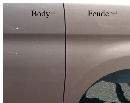
Fig. 1 Color mismatch example (In the production preparation stage).
